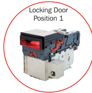
Cash Box: 300 Lockable (PA186) Door: Front Right (Standard)
